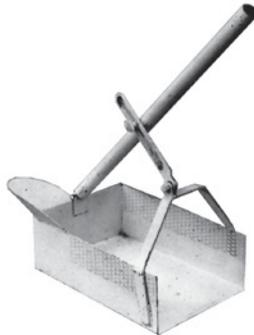
Figure 30 : Drague manuelle (type CEMAGREF)
